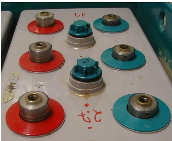
Fig. 18 Pole growth of OPzS cells at the end of life
