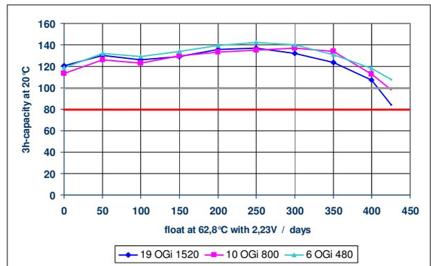
Fig. 14 OGi 3h-capacity within 425 days at 62,8°C
