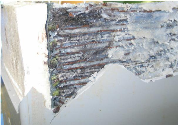
Fig. 11 OPzV2000 after 450 days at 62,8°C, Compression of the styropor block at the bottom
