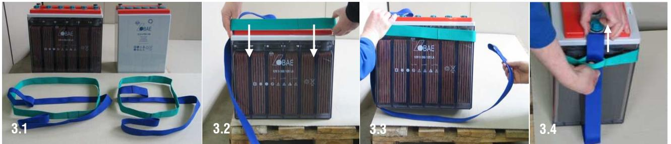
3.1 The block lifting device 385 (left) is for the large blocks (L = 380 mm), the block lifting device 280 (right) for the small blocks (L = 272 mm).
